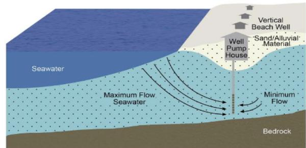
Figure 2 - Beach Well Concept for Water Supply to Plant
