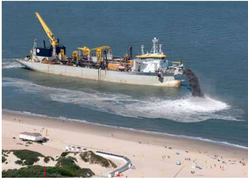
In Zeeland, the trailing suction hopper dredger Charles Darwin sprays on new sand to replenish the beach.
