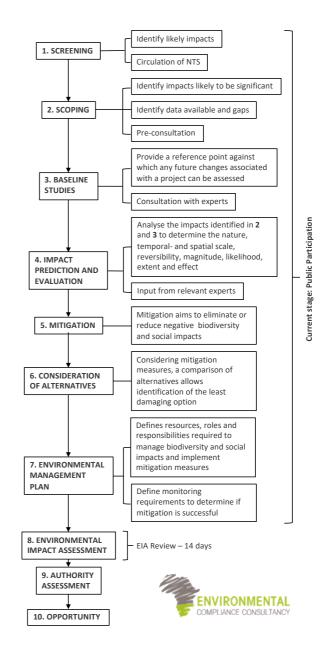
FIGURE 2 - FLOWCHART OF THE ENVIRONMENTAL ASSESSMENT PROCESS
