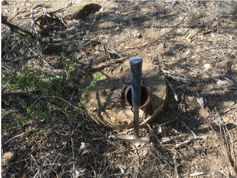
Old drill-site - drill-hole collar and uncapped Standpipe (1970's)
