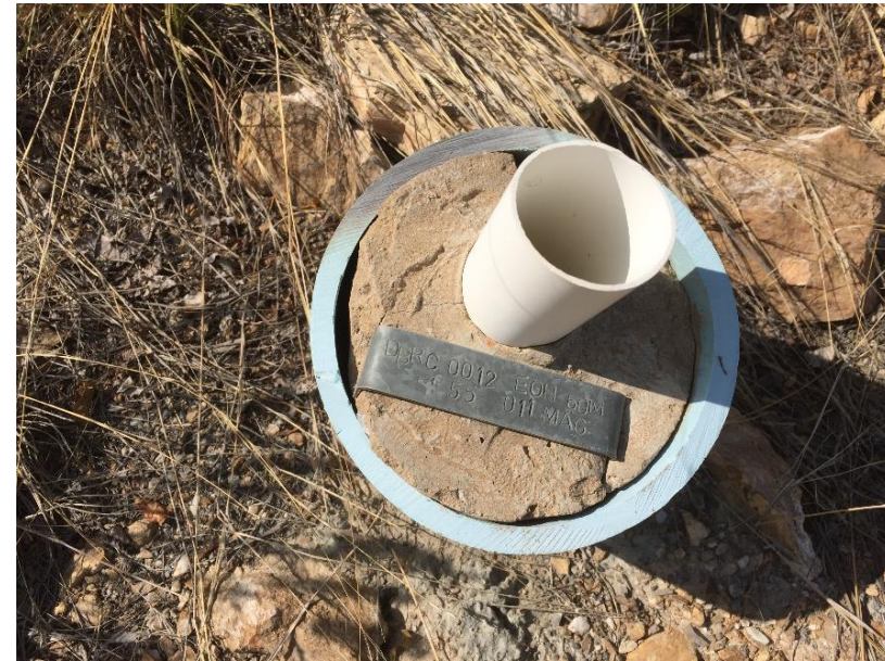
Recent RC drill collar - covered with loose concrete plug bearing RC numbers & details
