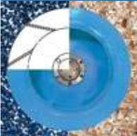
**Chip Impeller - Type S** The chip impeller is a closed, partly self-cleaning bladed impeller with straight, backward oblique blades. This impeller is used for transport of grinding and polishing dust, dry sawdust and shavings, etc. The chip impeller has an efficiency of up to 81%.
