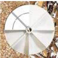
**Transport Impeller - Type T** The transport impeller is an open, self-cleaning bladed impeller with straight, radial blades. This impeller is used for transport of shavings, chips, etc. The transport impeller has an efficiency of up to 61%.
