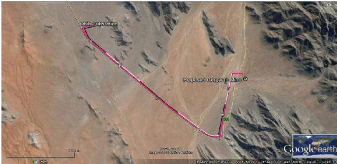
Figure 7: Suggested layout of alternating marked and unmarked sections of the proposed power line. Sections a, c and e should be fitted with alternating spirals and flappers, while sections b, d and f should be left without any devices. The total distance to be fitted with devices is about 4.7 km.
