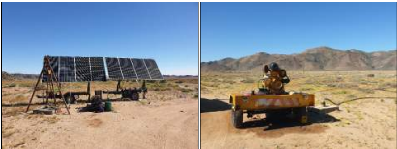
Figure 2-16 SolarBH (left) and GenBH (right) being pumped at \sim 3.5\text{ m}^3/\text{h} for use in drilling on site.
