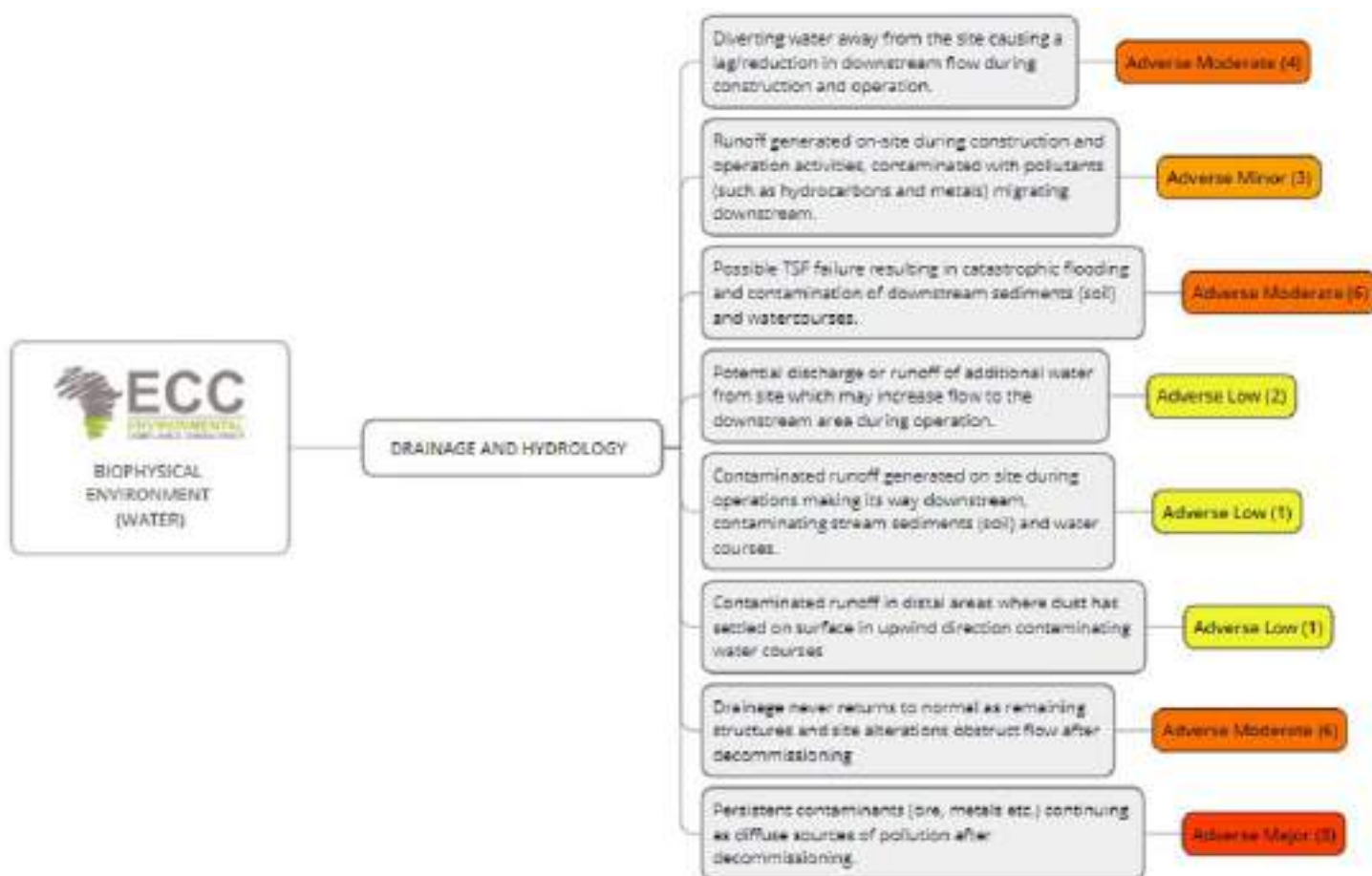
Figure 52 - Impacts of construction and operation activities on drainage and hydrology
