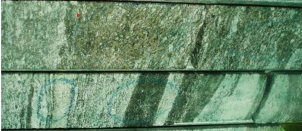
Figure 8 - Sawn NQ Drill Core showing the banded nature of the Omitiomire Ore.
