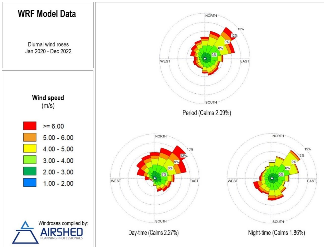
Figure C-1: Period, day- and night-time wind roses for the period 2020-2022 as obtained from the modelled WRF data
