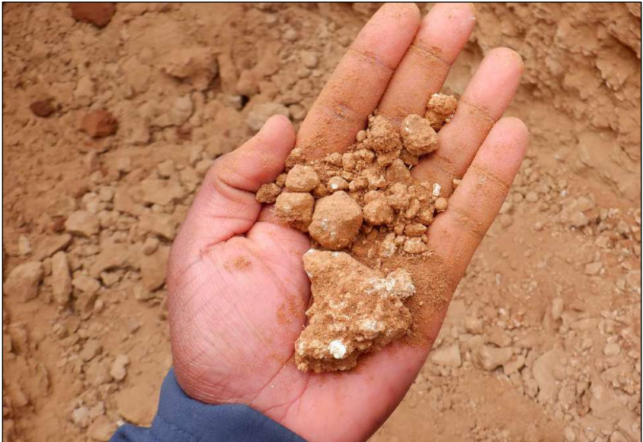
Plate 21: Zoomed in view of well-developed calcrete nodules of soft rock strength.
