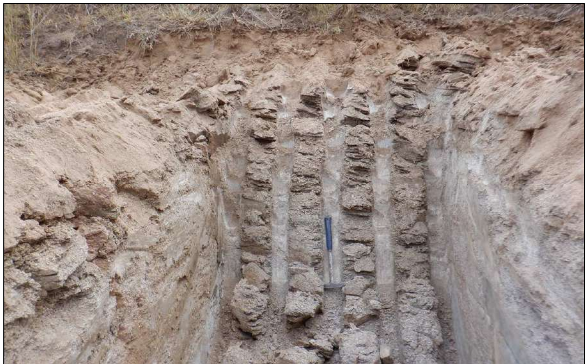
Plate 16: Shallow refusal on soft rock gneiss WRD-TP20.
