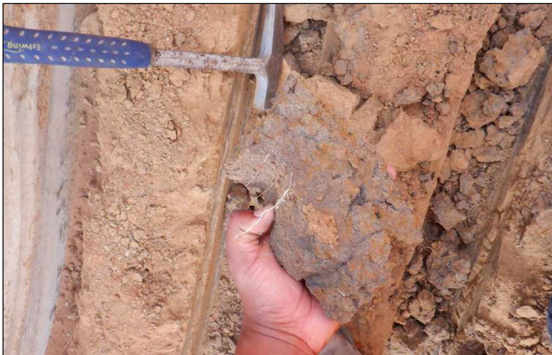
Plate 4: Zoomed in view of ferruginized soils at SWD-TP11.
