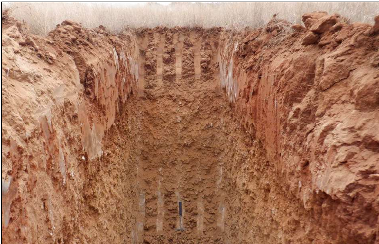
Plate 20: WRD-TP34 exposing well developed nodular calcrete horizon.
