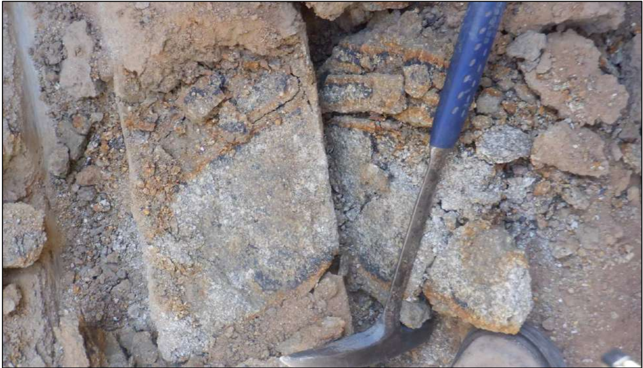
Plate 7: Refusal at HLP-TP06 on very dense residual gneiss.
