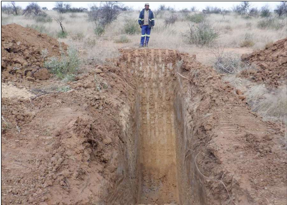
Plate 15: Typical pedogenic profile with refusal on medium hard rock gneiss.
