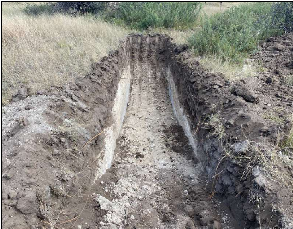
Plate 18: Shallow refusal on hardpan calcrete of soft rock strength at WRD-TP23.
