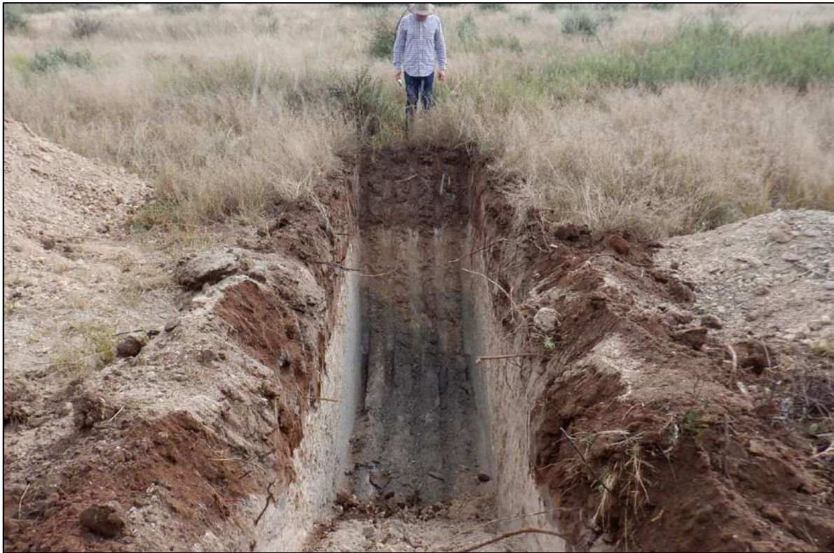
Plate 5: Shallow refusals encountered on soft rock gneiss at SWD-TP25.
