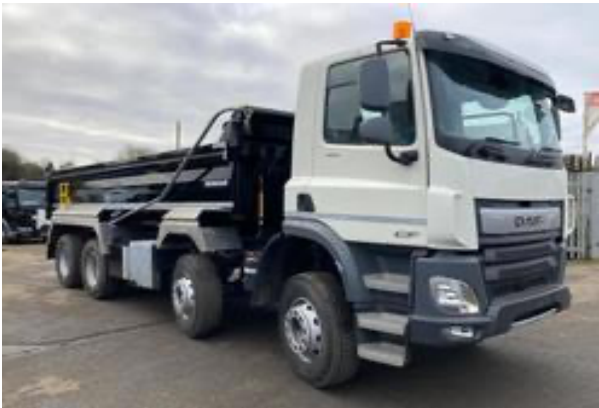
Figure 15 DAF CF 450 8x4 32 Tipper fitted with a Fruehauf Muck-Away Tipper body.
