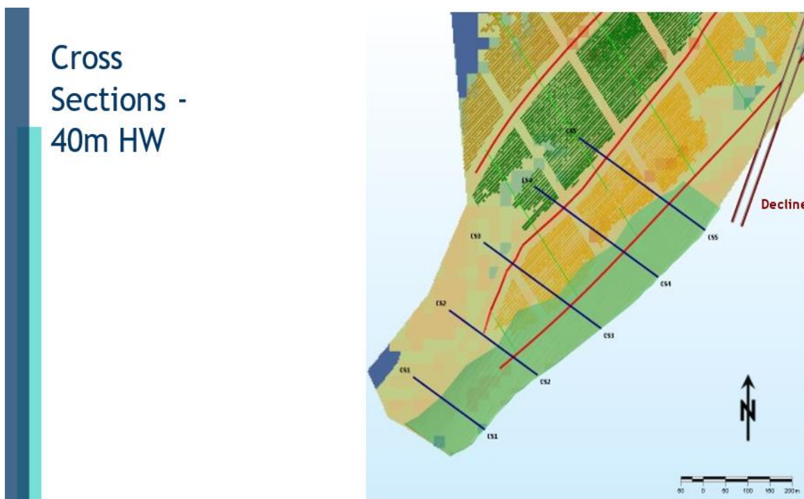
Figure 7 – Proposed site layout showing mining areas (Central shoot open pit), with 40 m high walls and indicated mining cross sections (Source: Practara).
