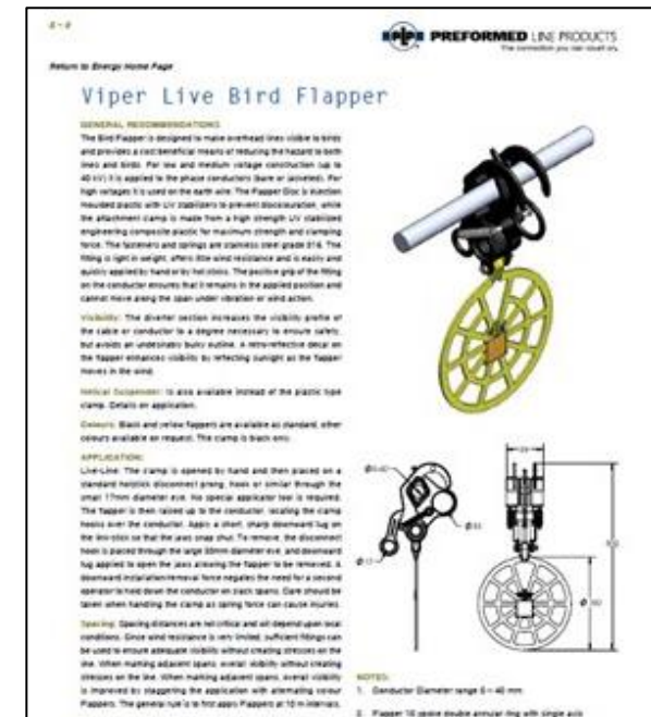
Figure 29. Example of power line marking device: Viper Live Bird Flapper (Viper), used as a mitigation for bird collisions (made in South Africa).
