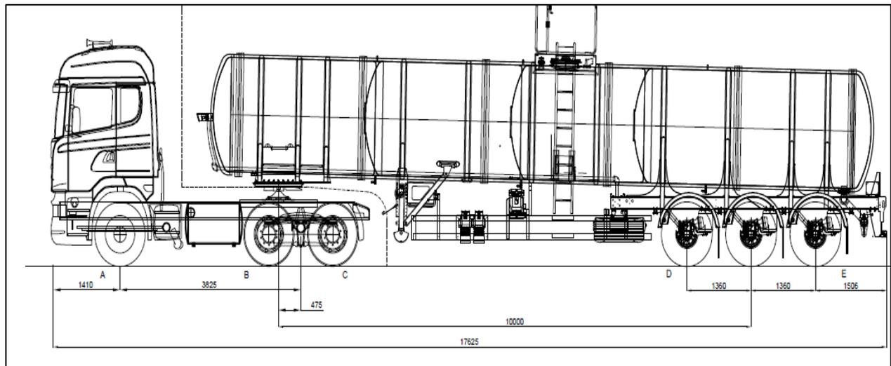
**FIGURE 3 - ILLUSTRATION OF THE PROPOSED PROJECT'S TANKER TRUCKS**
