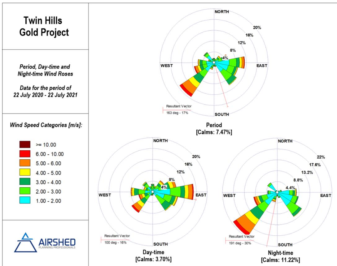
Figure 4: Period, day- and night-time wind roses based on Twin Hills on-site weather data (23 July 2020 – 22 July 2021)
