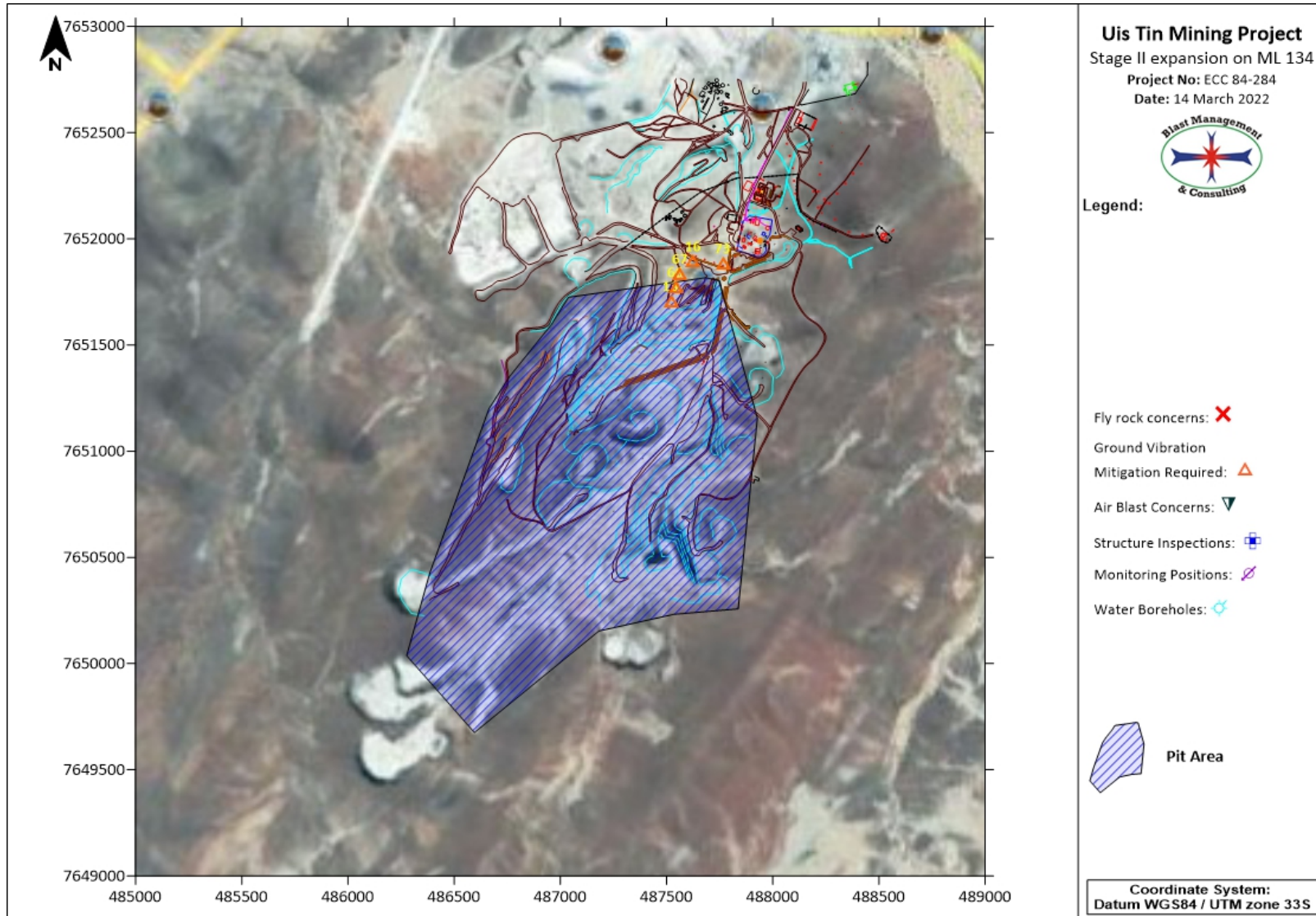
Figure 24: Structures identified where ground vibration mitigation will be required.
