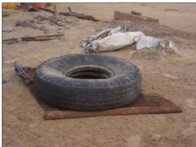
FIGURE 8 - APPARATUS OF THE TYRE AND GRID USED TO LEVEL GROUND TRACK CLOSURE IN NAMIBIA (MANSFELD, 2006)
