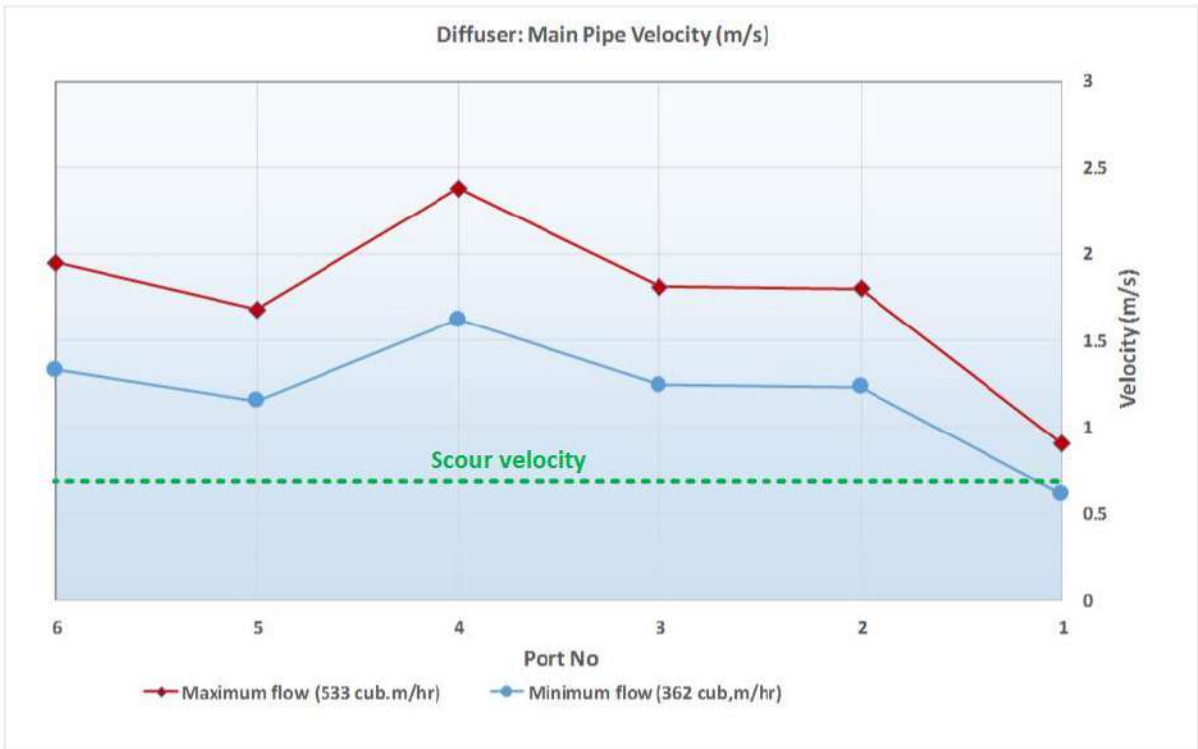
Figure 14: Diffuser Hydraulics: Main Pipe Velocities
