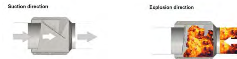
FIGURE 10: ILLUSTRATION OF THE FIRE CONTROL SYSTEM WITH A BACK-PRESSURE FLAP VALVE. SOURCE: ENVIROX, 2020
