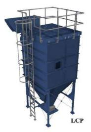
"All LCP Ex, LCP units have generously sized integral pre- separation chambers to increase their dust load capacity whilst reducing the load on the filter cartridges. Maintenance is from the top, within handrails if specified. A range of space saving integral fans from 5,5 kW to 18,5 kW may be specified, with optional air silencers. Larger units may be served by floor mounted high efficiency Combi-fab fans".
