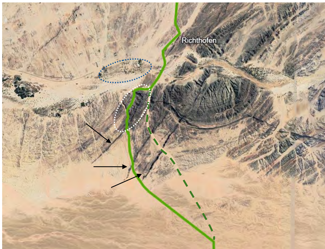
Figure 34: The Richthofen pipeline section with proposed route change. Important habitats along this route include the Swakop River with open surface water and bird habitat (blue dotted oblong); dolerite ridges (black arrows) and rocky areas (white dotted oblongs). The dark green dashed line indicates the original pipeline route.
