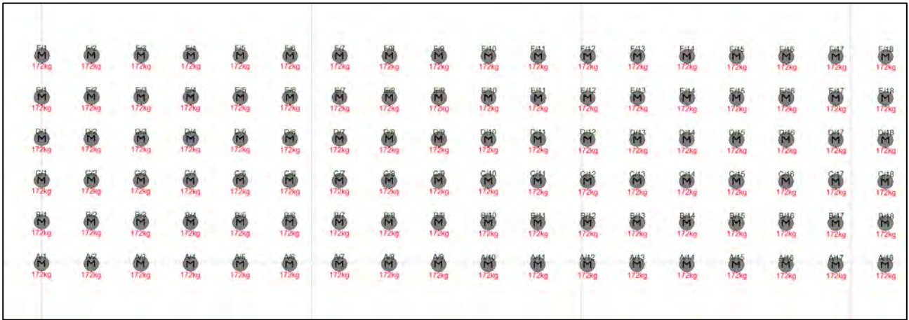
Figure 8: Blast holes layout with charge mass per blast hole
