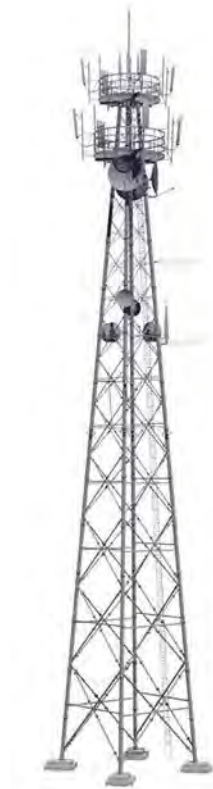
Figure 3 - A typical sketch of a lattice telecommunication tower
