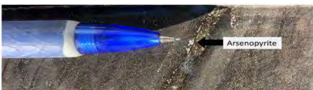
Arsenopyrite in cm scale veinlet in schist
