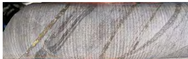
Cm-scale quartz sulphide veins in schist
