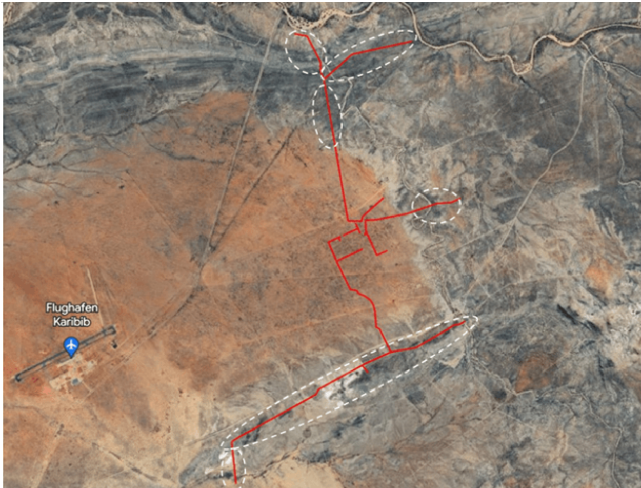
Figure 96 - Various 11 kV overhead transmission lines and areas indicated (white dashed) where flight diverters are to be installed (Source: (Cunningham, 2023)).
