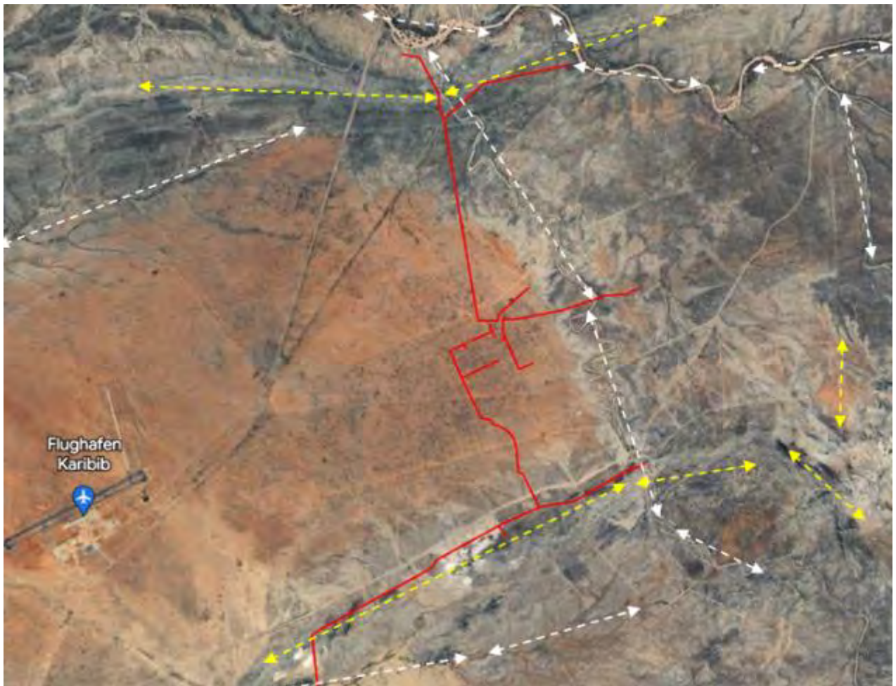
Figure 98- Expected bird flight paths along ephemeral drainage lines (white dashed arrows) and between mountainous areas (yellow dashed arrows) in the general area. The 11 kV power lines are indicated by the solid red lines (Source: (Cunningham, 2023).
