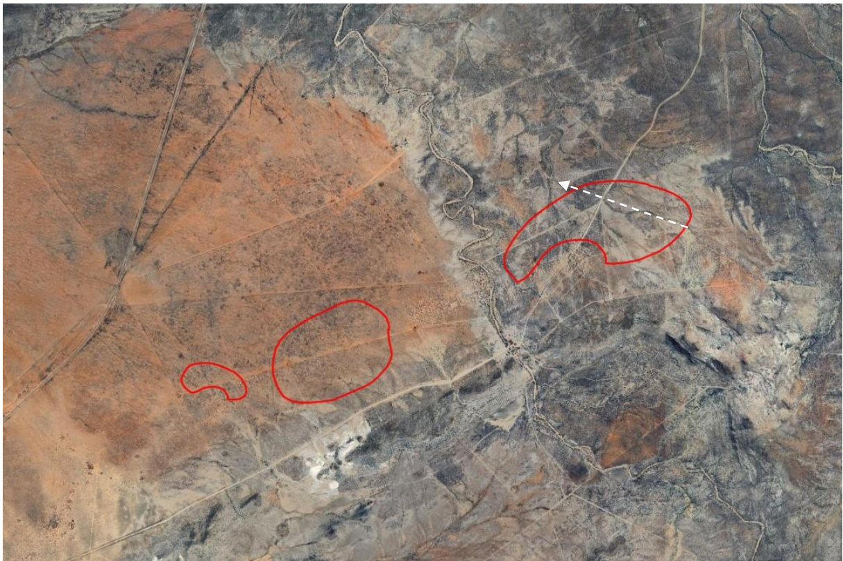
Figure 2. Waste Rock Dump (WRD) sites. White arrow indicates tributary to be avoided.
