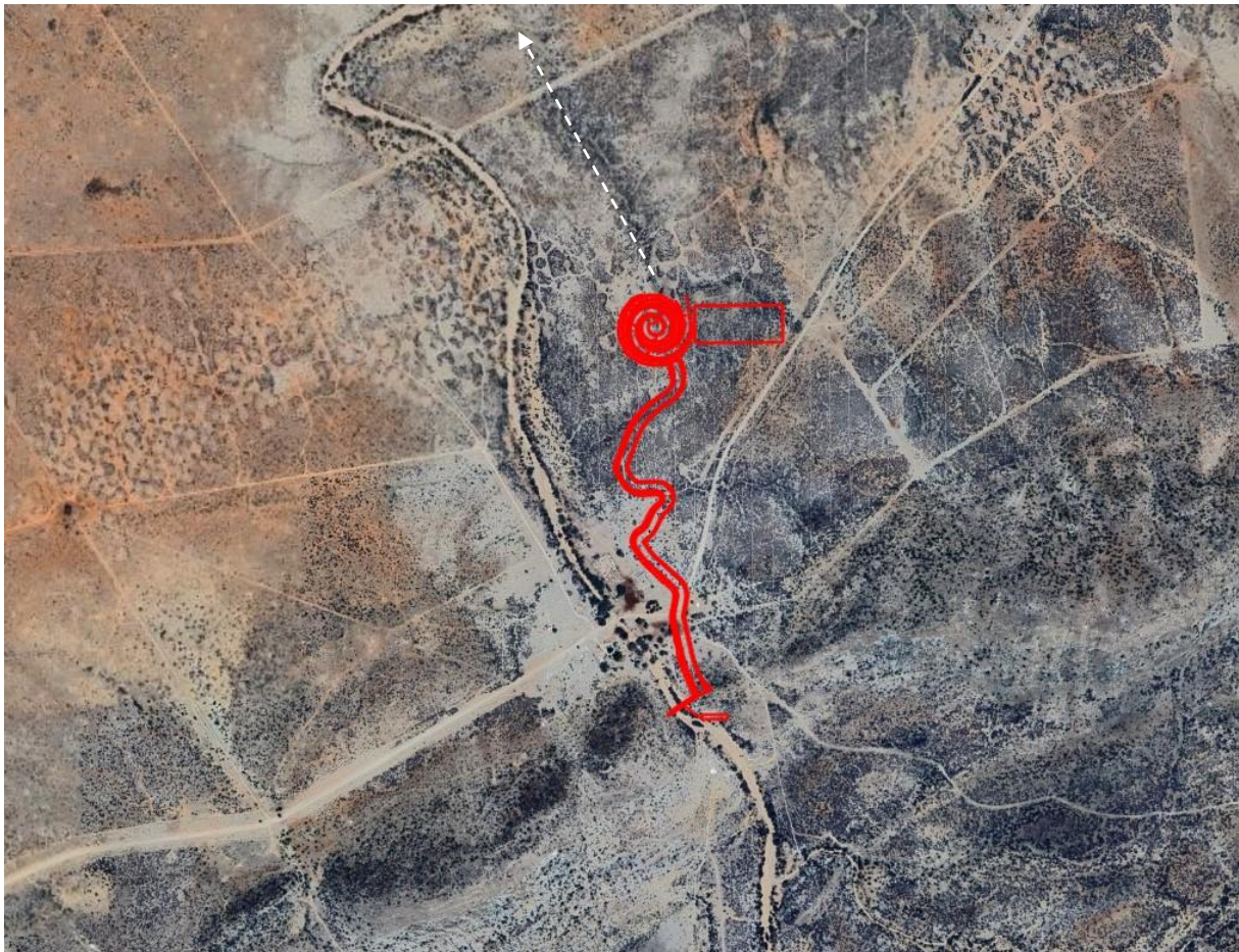
Figure 12. Okawayo River diversion and embankment dam site. The white dashed arrow indicates the proposed direction of flow of the Okawayo River rather than damming it into the proposed holding dam.
