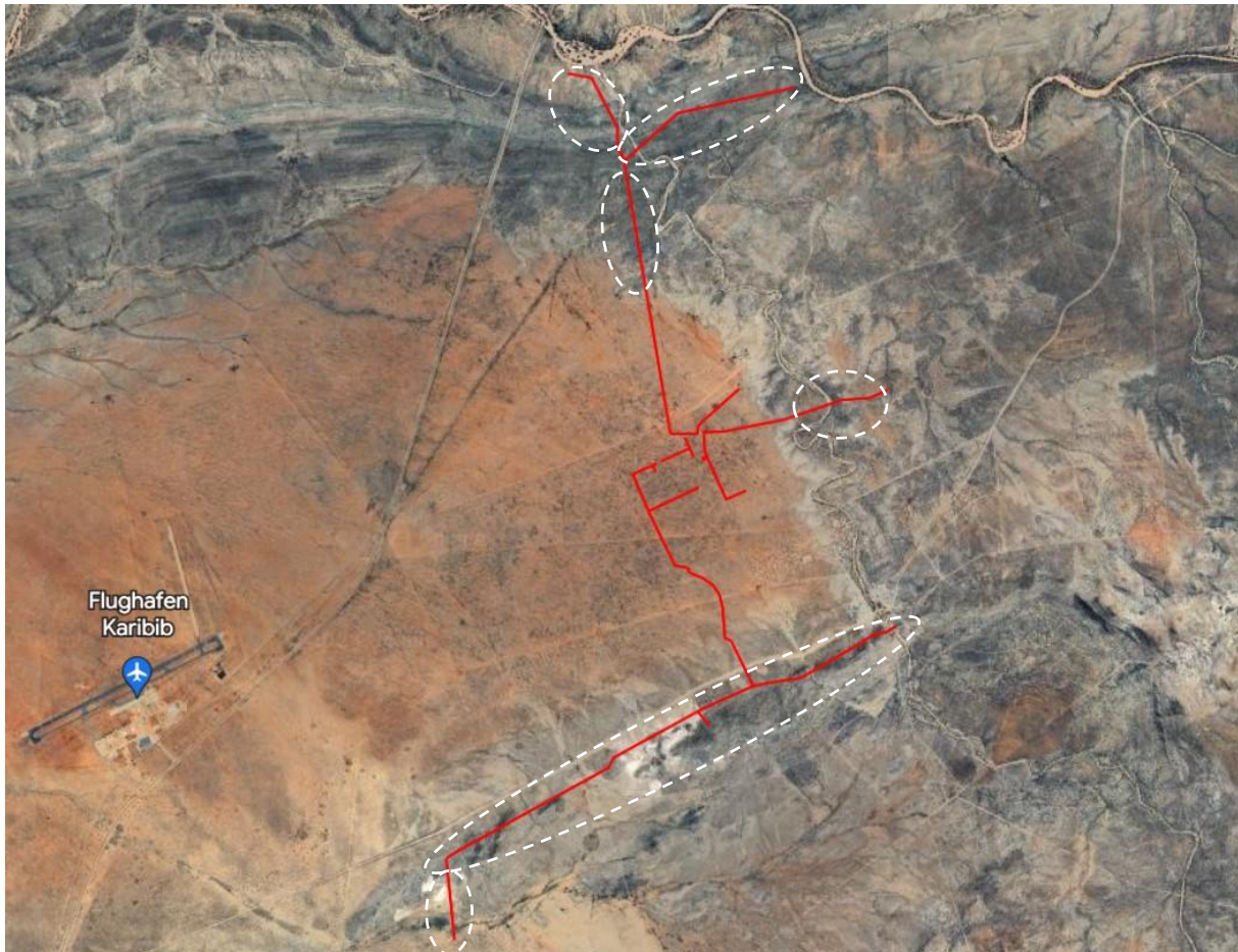
Figure 11. Various 11 kV overhead transmission lines and areas where flight diverters should be installed.
