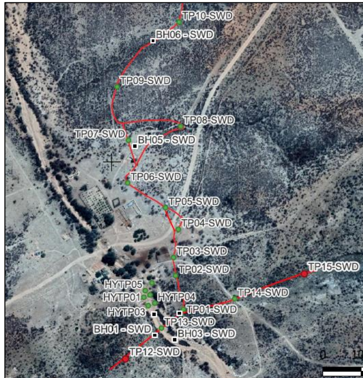
Figure 4-8: Layout of Test Pit and Borehole Positions.
