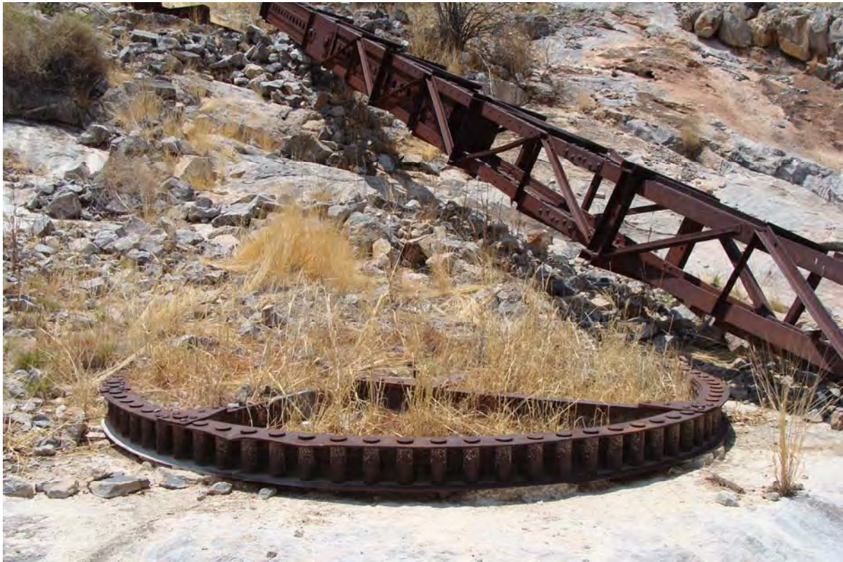
QRS 114/6 Dernberg marble quarry; base and derrick of rotating crane
