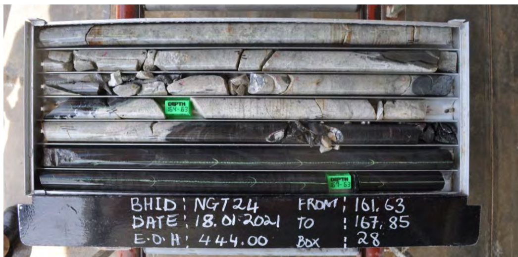
Photo 2-6: Fractured zone NGT24
