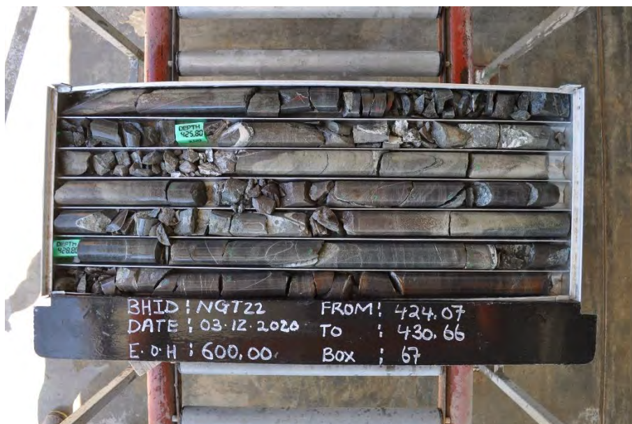
Photo 2-4: Low RQD and fracturing NGT22
