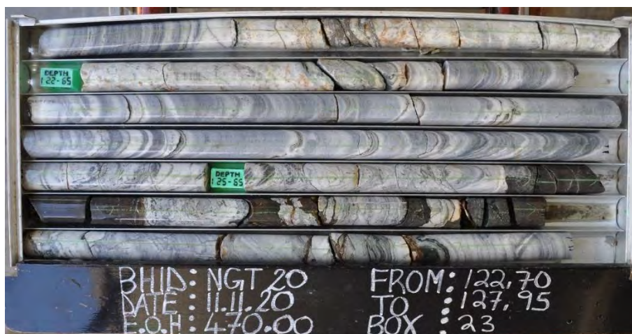
Photo 2-1: Typical Test Zone Across a Fault Breccia NGT20
