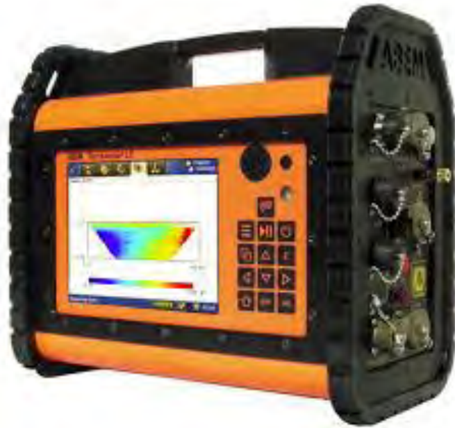
Figure 3: ABEM Terrameter LS2 Resistivity system
