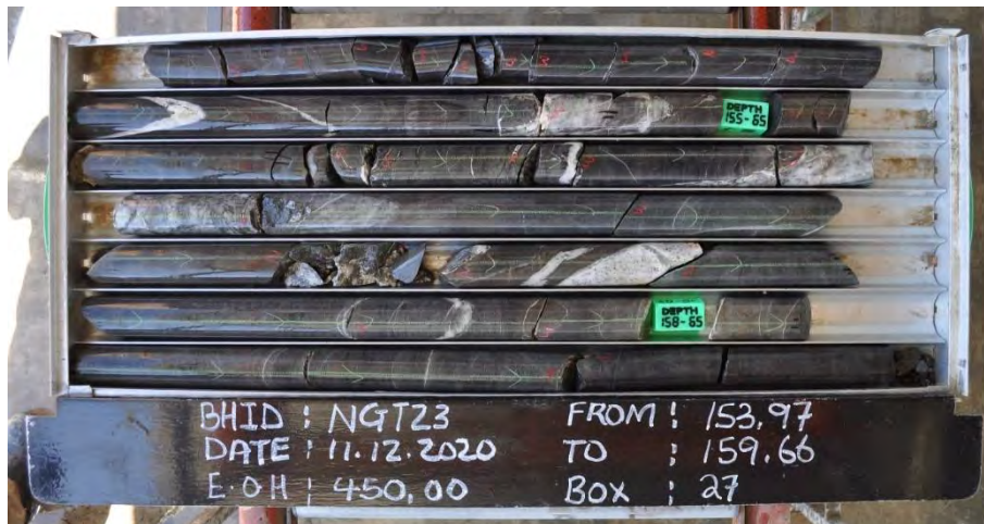
Photo 2-4: Fractured zone NGT23
