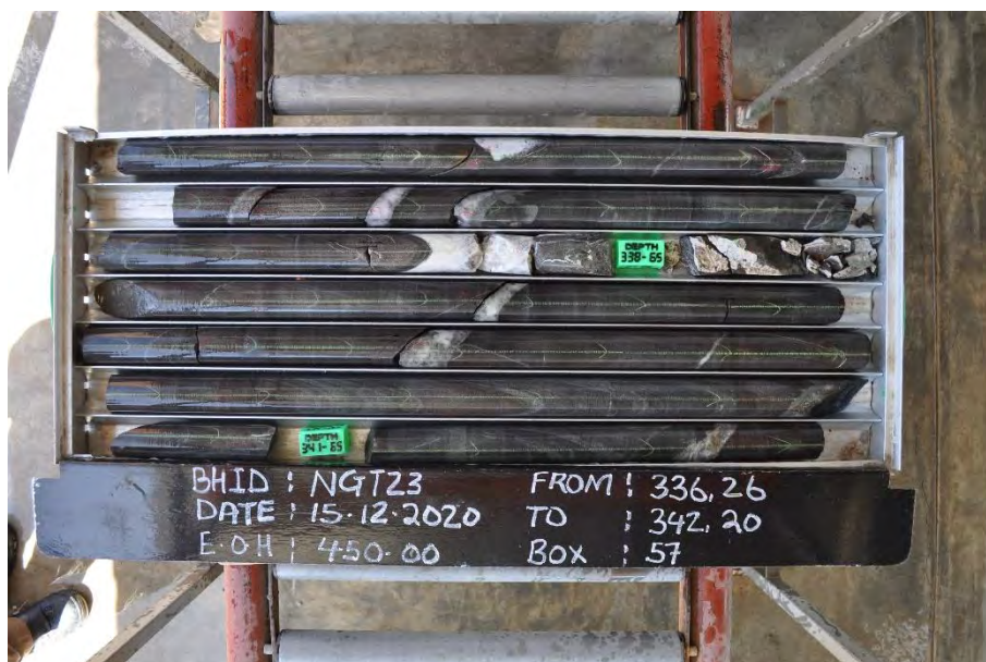
Photo 2-5: Typical test zone across a shear/fractured zone NGT23
