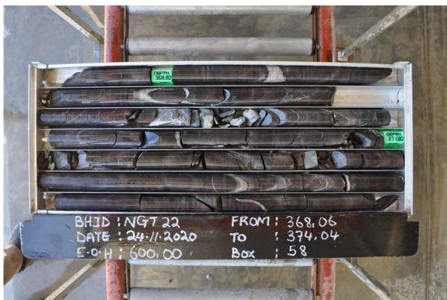
Photo 2-5: Typical test zone fractured shear NGT22
