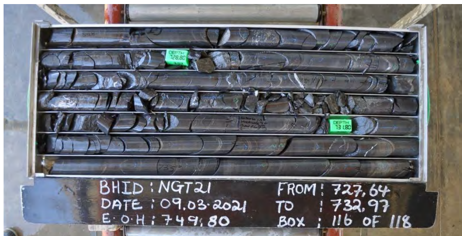
Photo 2-3: Typical test zone across a fracture – NGT21
