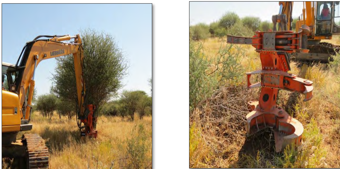
FIGURE 4-5: HYDRAULIC GRAB AND CUTTER USED IN LARGE SCALE FELLING (GIZ, 2015)
