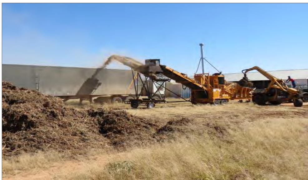
FIGURE 4-8: CHIPS TRANSFERRED ONTO A ROAD TRAILER (GIZ, 2015)
