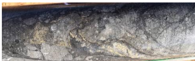
Brecciation and silicification in quartzite
